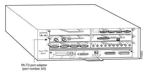
Figure 8-1 Serial Port Number Example—Cisco 7206
